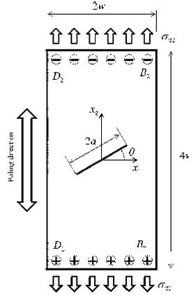
Figure 2: Inclined crack in a rectangular magneto-electro-elastic plate
