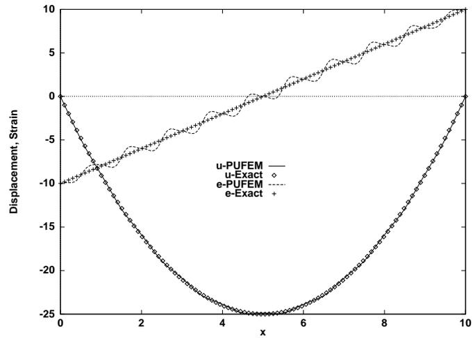
Figure 3: Results for  $d_{max} = 1.0$  with linear basis on the interior nodes (non-shifted basis)
