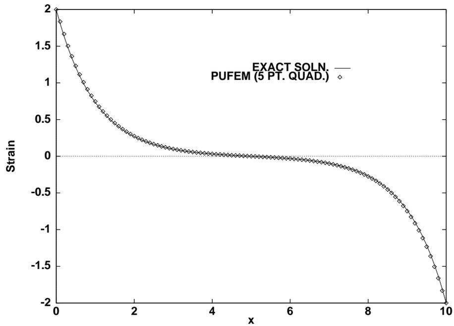
Figure 9: Strain along the 1D bar for example 4
