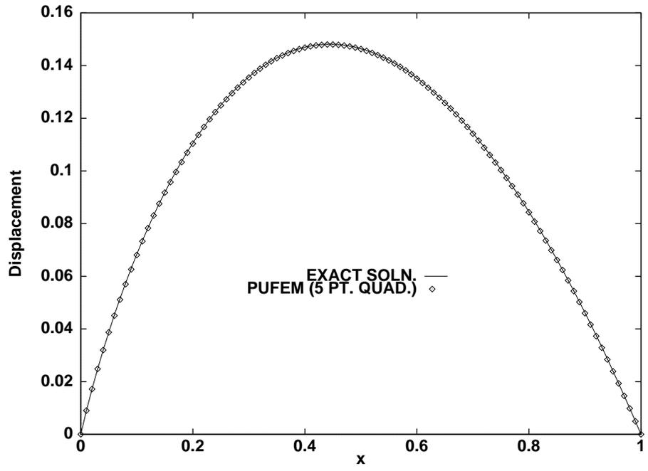
Figure 4: Displacement along the 1D bar for example 2
