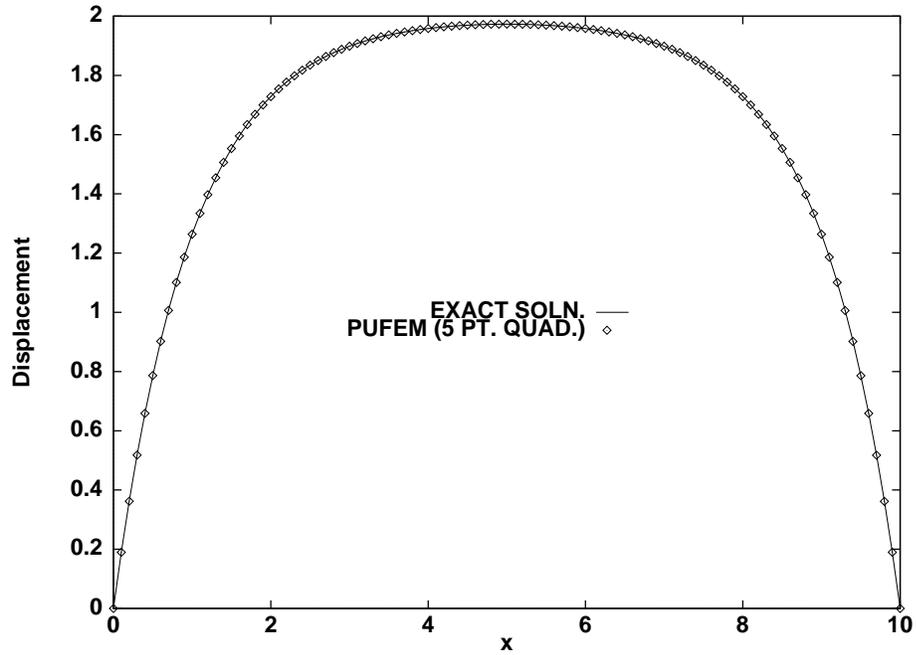
Figure 8: Displacement along the 1D bar for example 4
