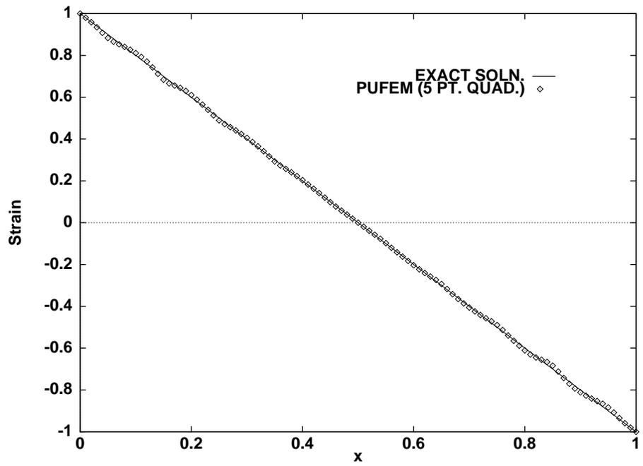
Figure 3: Strain along the 1D bar for example 1
