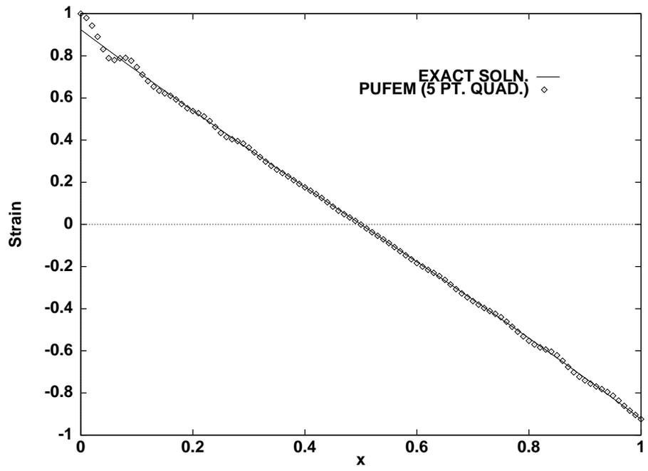
Figure 7: Strain along the 1D bar for example 3
