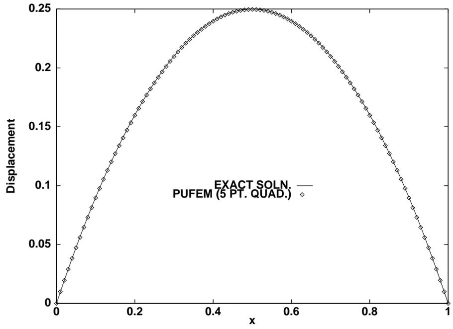
Figure 2: Displacement along the 1D bar for example 1
