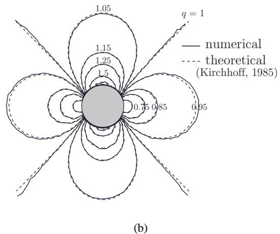
**Figure 10** : Potential flow past cylindrical inclusion. (a) Mesh; and (b) Isocontours of flow rate  $q$
