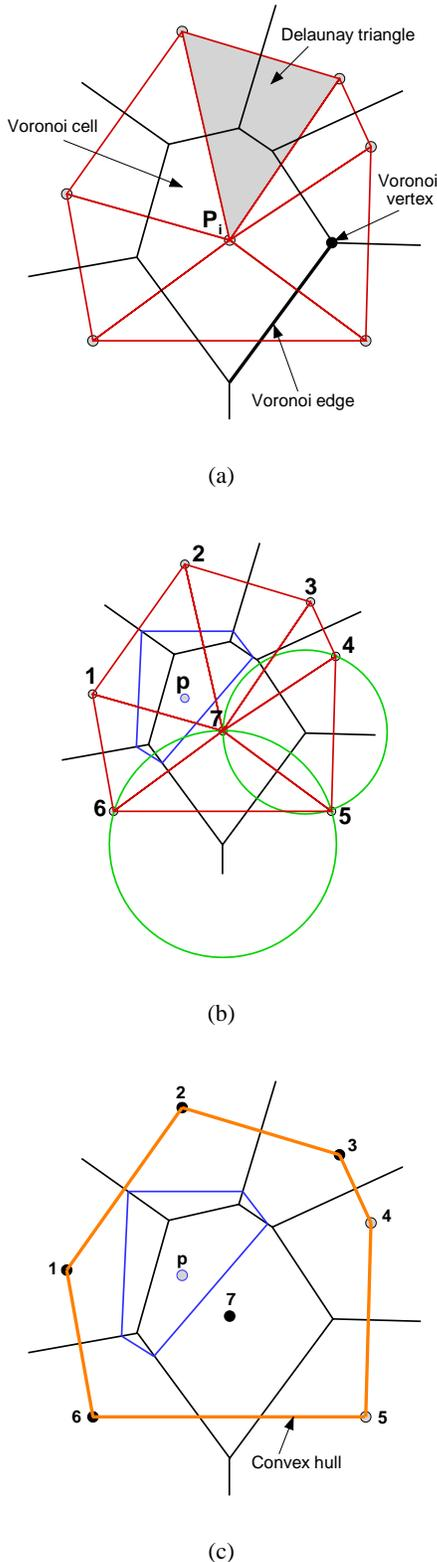
**Figure 1** : Geometric constructs. (a) Voronoi diagram and Delaunay triangulation; (b) Delaunay circumcircles; and (c) Natural neighbors (filled circles) of point  $p$ .
