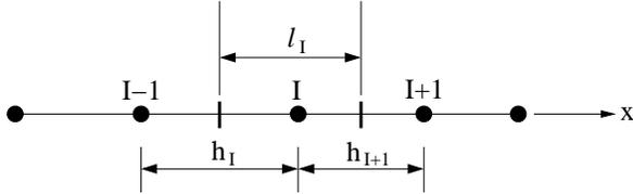
**Figure 4** : Voronoi cell for a non-uniform grid in 1-d.
